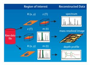
Concept of retrospective analysis from the stored raw data file. Spectra, images, and depth profiles can be reconstructed from any area at any depth and from any ion.
