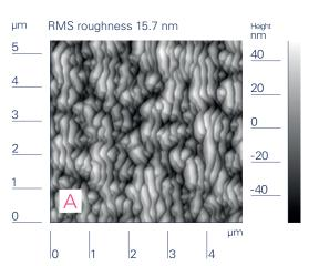
Contact AFM image measured at position A in the surface profile above.
